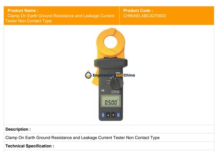
Clamp - On Earth / Ground Resistance & Leakage Current Testers: Clamp - On Earth / Ground Resistance and Leakage Current Tester (Non Contact Type) with Range : 0.025W-1500W, 0.300mA-30.00A AC, Data Logging, Data Hold, Programmable HI - LO Alarm, Autoranging and Auto Power Off functions. Jaw Opening : For Earthing Wire of 23mm Diameter
